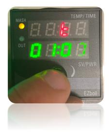
Pressing the knob in one time will display **dtSP**. The **dtSP** setting is at what temperature you want the timer to start at.
