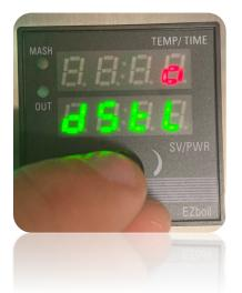
the display reads **dStL**. This will allow you to adjust the level of the heating element on a scale of **1 to 100**.
