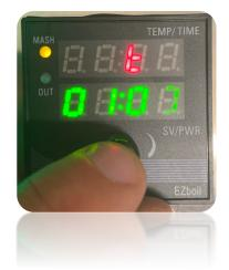
Pressing the knob in one time will display **tSP**. The **tSP** setting is at what temperature you want the timer to start at.
