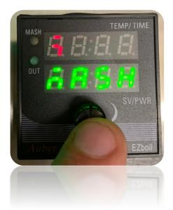
In order to set the controller to pre-heat mode, press in the knob for the display to read **ñASH**. The controller will now be in pre-heat mode. This will allow you to adjust the controller to a particular set temperature by rotating the knob clockwise for **UP** and counter clockwise for **DOWN**.
