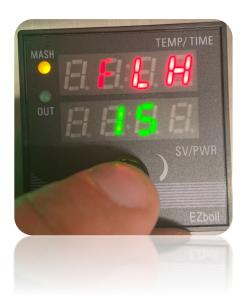
Pressing the knob in again will display **Eo**. The **Eo** setting is if you want the heating to continue or stop at the end of the timer. Set **Eo** to **ON** if
