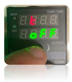
Pressing the knob **2 times** will display **tdlr**. In this setting, **dn** will count the timer **DOWN** and **up** will count the timer **UP**.
