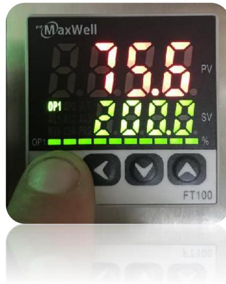
**Step 2: The controller is pre-set with a run time of 18hrs or 1080 mins.**
